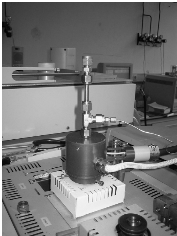
Fig. 1. GSG Pyromat with modified pyrolysis chamber and sample probe.
